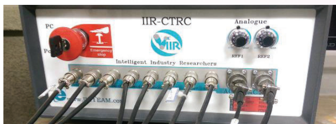
Figure 1: New closed loop control system of the cyclic triaxial device
