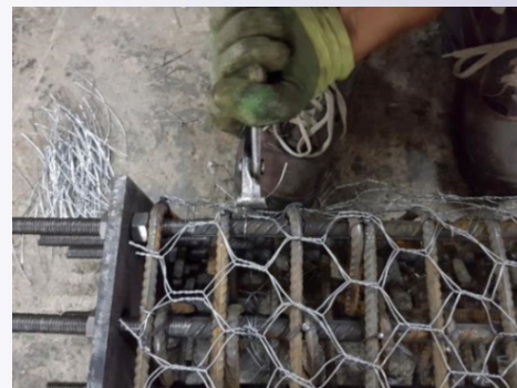
Figure 1: Fabrication of RC columns confined by HCW
